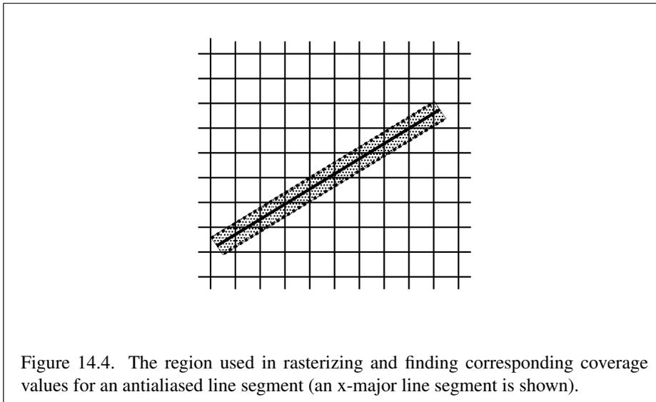
Figure 14.4. The region used in rasterizing and finding corresponding coverage values for an antialiased line segment (an x-major line segment is shown).
