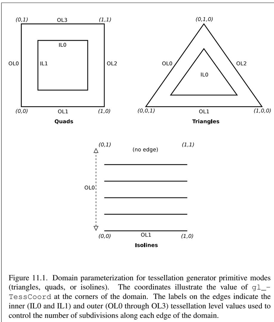
For `quads`, all four outer levels are relevant. For `triangles` and `isolines`, only the first three or two outer levels, respectively, are relevant. Negative inner levels will not cause a patch to be discarded; they will be clamped as described below.
