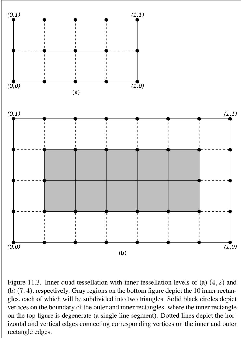
passed to subsequent pipeline stages and the order of the vertices in those triangles are both implementation-dependent. However, when depicted in a manner similar to figure 11.3, the order of the vertices in the generated triangles will be either all clockwise or all counter-clockwise, according to the vertex order `layout` declaration.
