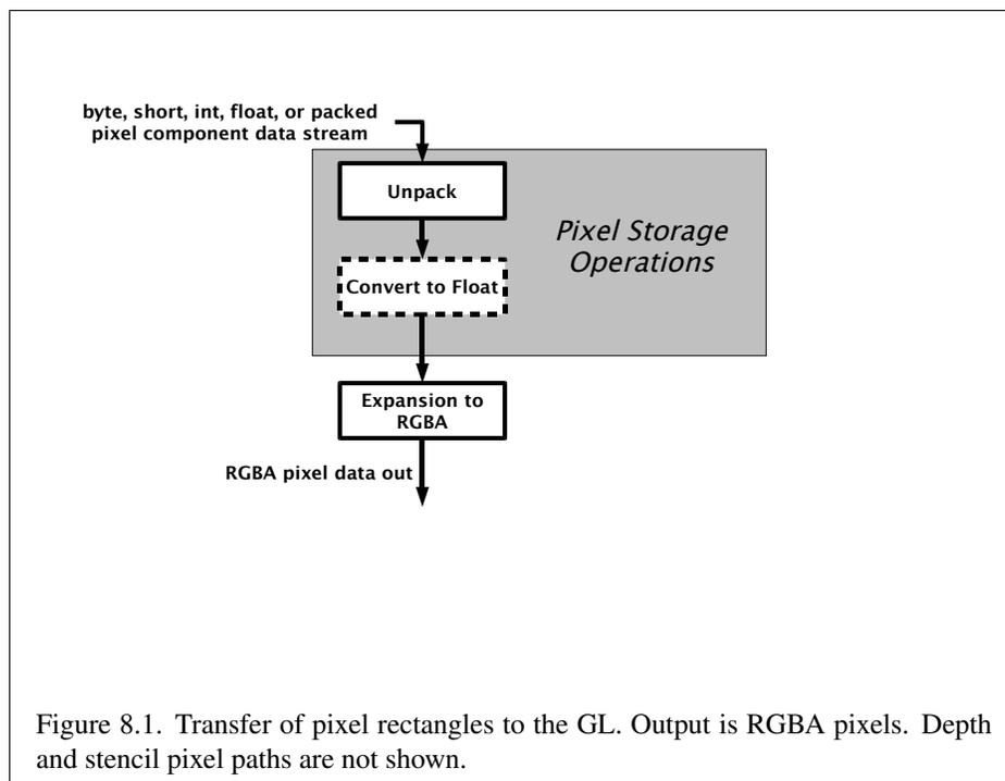
Figure 8.1. Transfer of pixel rectangles to the GL. Output is RGBA pixels. Depth and stencil pixel paths are not shown.
